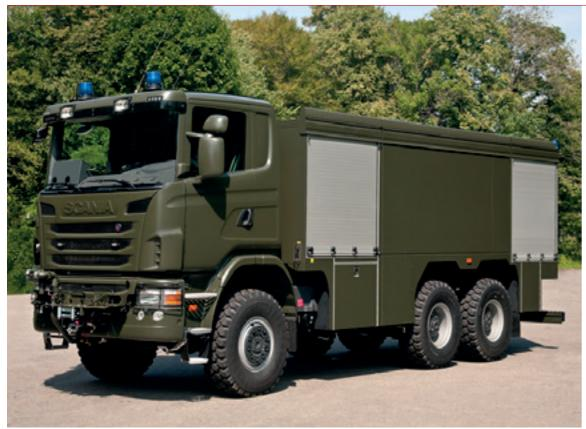
frame that eliminates stress resulting from the movement in rough terrain. Block construction consists of a specially designed subframe made of three components: equipment compartment + extinguishing tanks + pump compartment, each of them is independently mounted on the flexible elements on the subframe.
