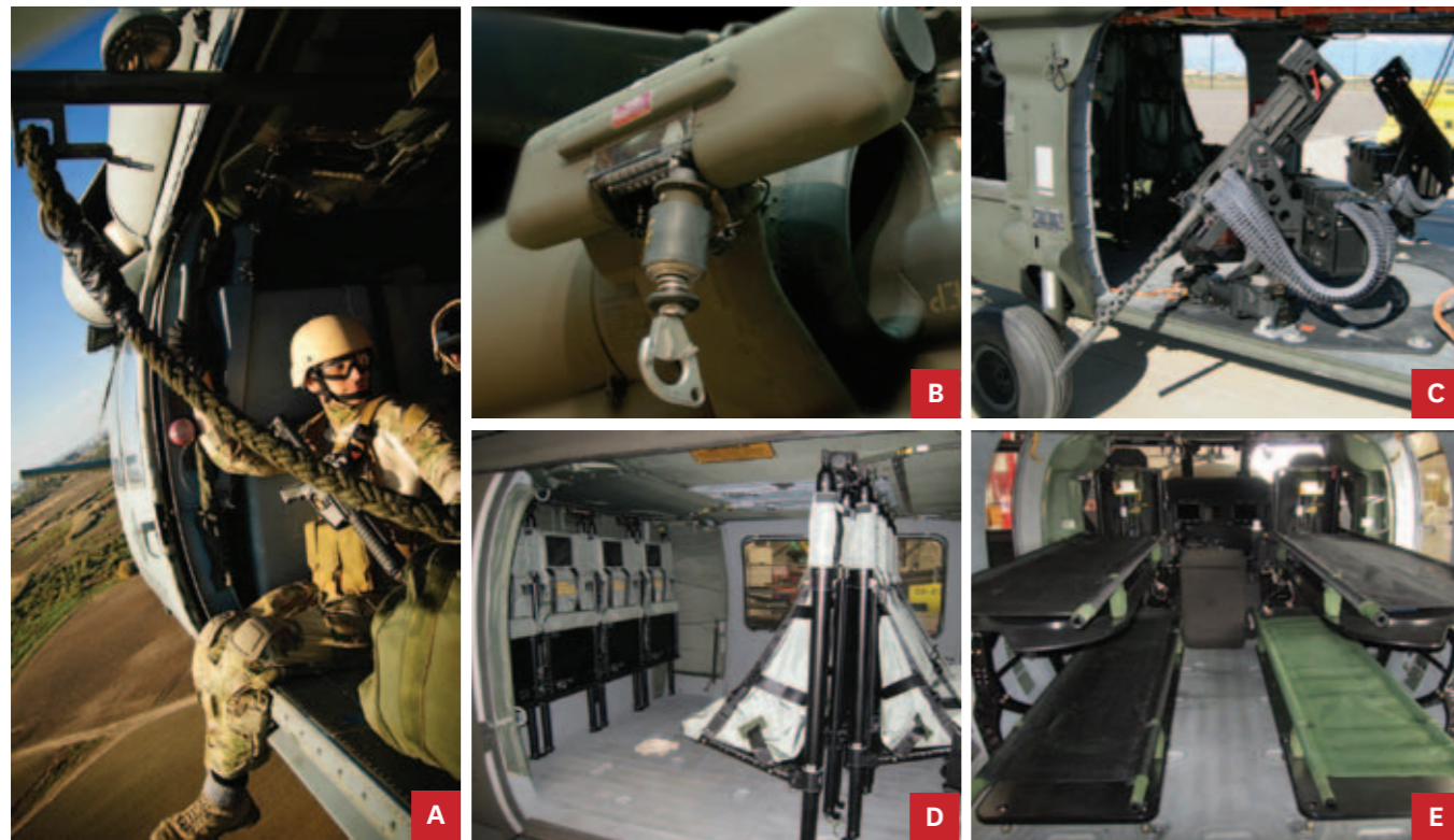
A. Optional FRIES Bar B. Rescue Hoist (enhanced utility configuration) C. Optional Interior Gun Mount (M3M .50 cal shown) D. Folding Troop Seats (optional) Improve Use of Floor Space E. Optional 4-place Interior Litter System
