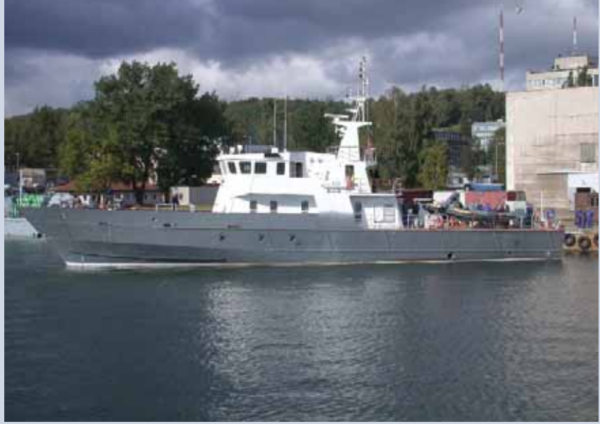
Profile view of the NS-935 type fast patrol craft. Note the fast inspection boats stowed at the stern of the vessel.
