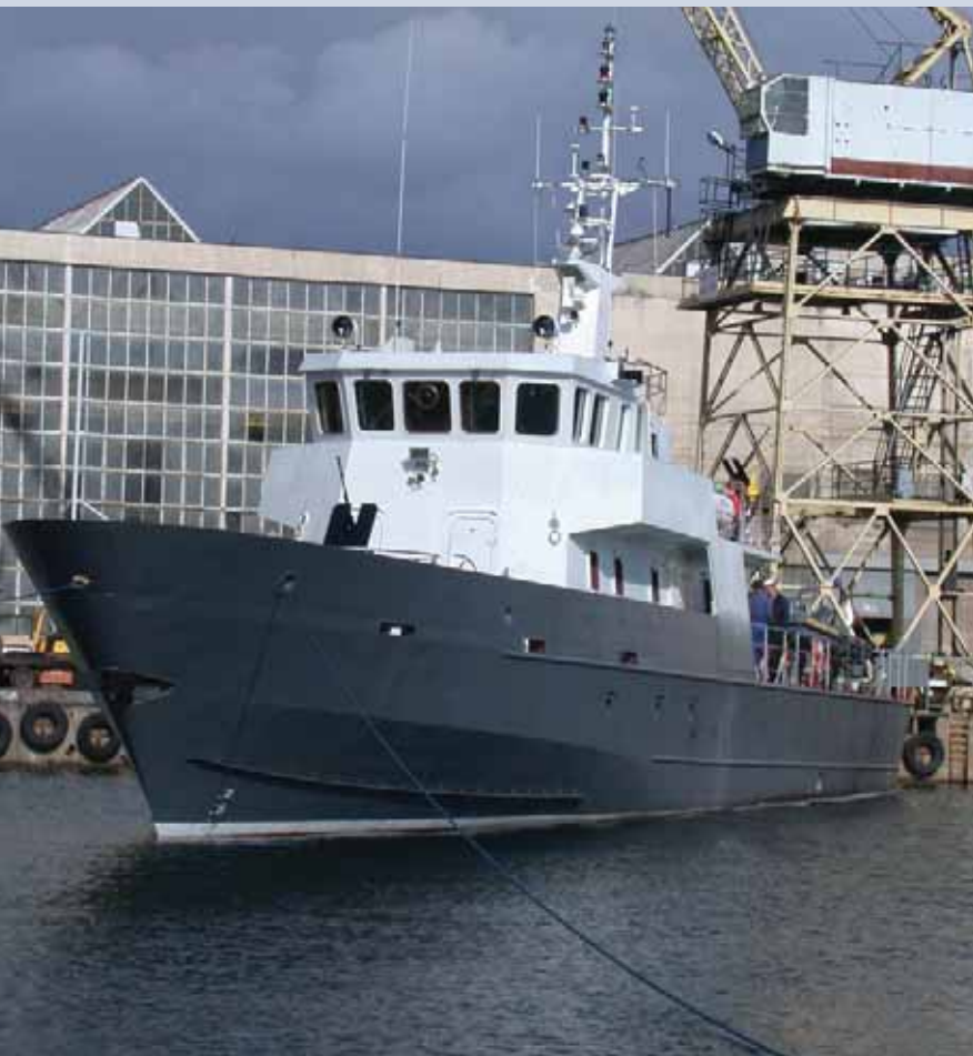
NS-935 type fast patrol craft for Indonesia pictured during the dock trials. Please note the hull shaped for speed and the wheelhouse with good round visibility.
