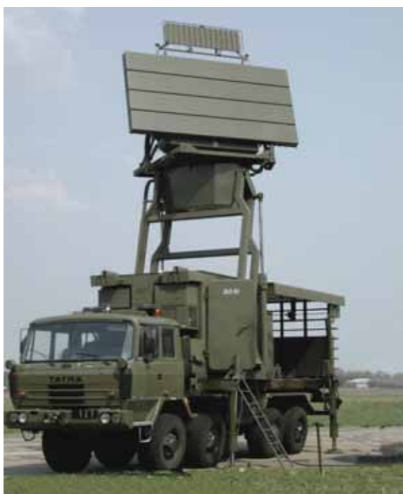
TRS-15/TRS-19 Mobile Medium Range 3D Surveillance S-Band Radar
